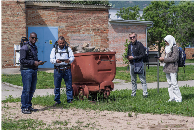
Fig 4: A team performs surface screening measurements with backpack detectors to find out the spatial distribution of the radioisotopes
