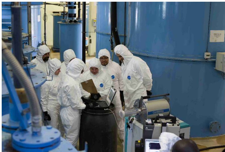
Fig. 3: Gamma spectrometry measurements performed inside a yellow cake production facility
