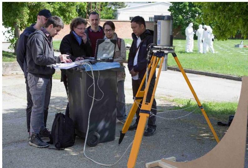
Fig.1: Field calibration of a high resolution gamma spectrometer.
